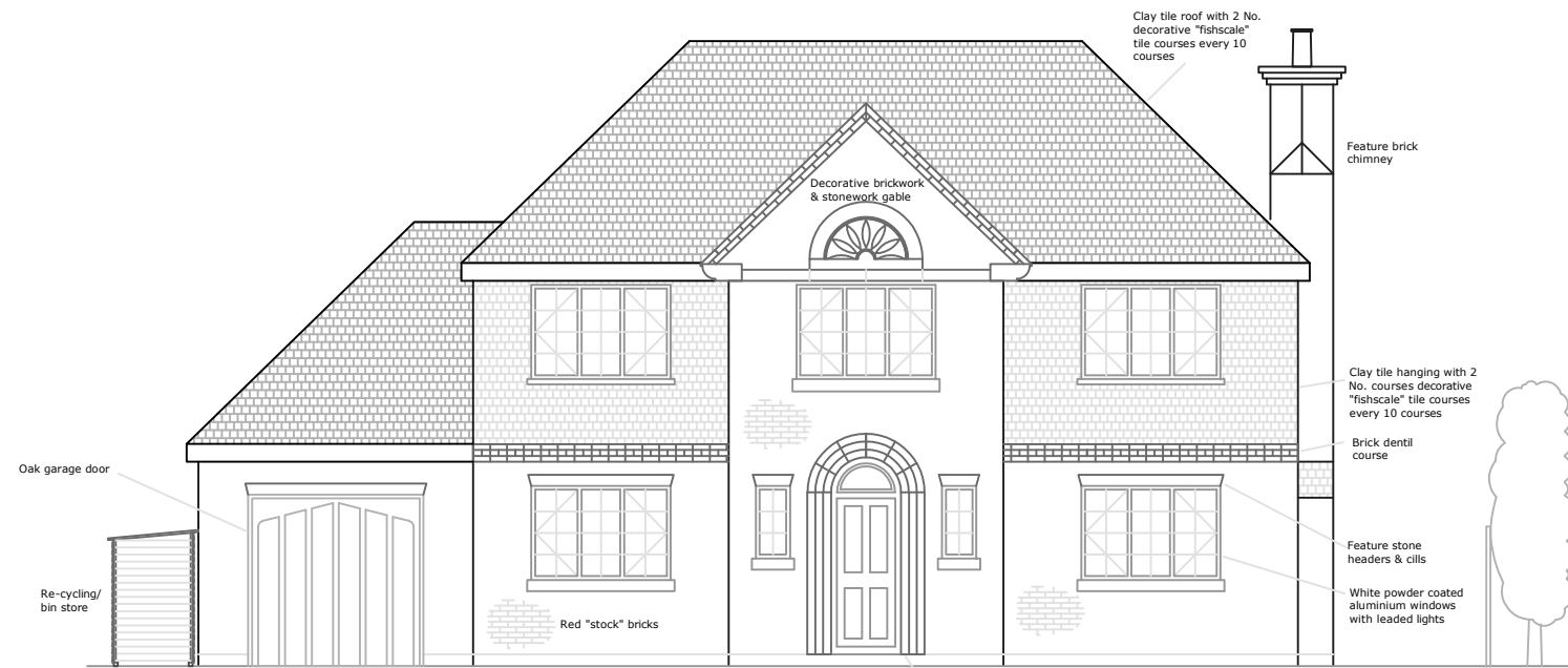
Front Elevation (View from Derrydown)
